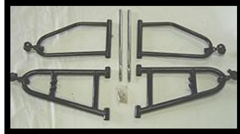
YFZ 450 A-Arms Shown in bare metal +2"/+1" configuration. $460.00
