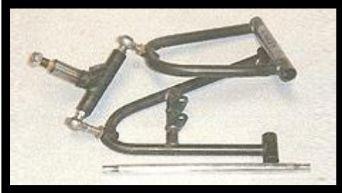
Banshee A-Arm / spindle combo Lightest weight, smooth track only.
