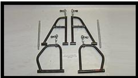
Banshee Drag A-Arms Extends wheel base forward to keep weight on rear tires. Image shows +0" / +3.5" (Total weight of all parts in photo is 8 lbs.) $460.00
