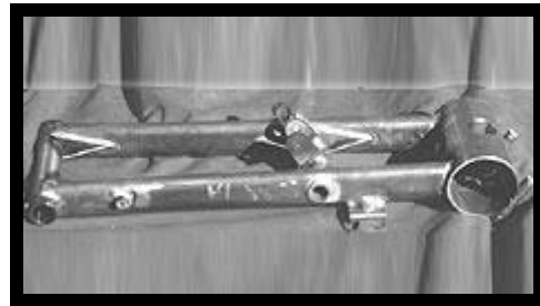
'88-89 250R Swingarm Shown in bare metal. Oval tube model. (Square tube also available) $429.00
