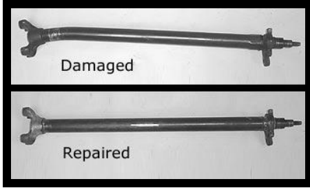
Steering stem repairs Bent steering stems repaired with chromoly. $70.00
